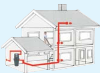
Fig. 1 Positioning the vacuum unit
